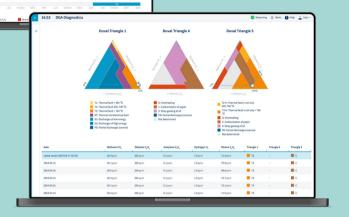
DGA diagnostics tools such as Duval's triangles. Measurement data can be quickly exported in csv format for further analysis, and alerts and alert levels can be set and customized directly from the interface. What's more, no clientside software installation is needed.
